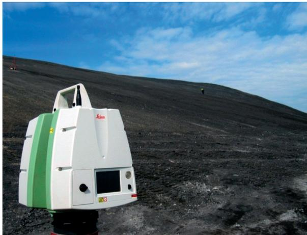
Fig. 3. The used TLS device during the course of the survey (Geo S.T. OÜ 2012)
