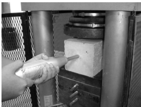
Figure 2 Schematic view for measurement of rebound number
