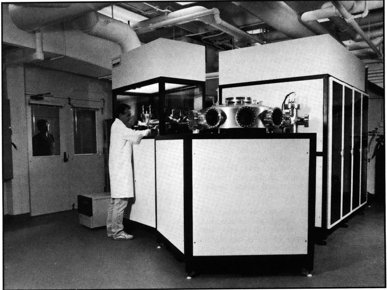
The system shown is a modular chemical beam epitaxy facility for the epitaxial growth of compound semiconductors. Research Specialist Steven C. Shepard places a sample into the ultra high vacuum introduction chamber, while Visiting Scientist Dr. Hidehito Nanto considers the layout of the growth reactor contained in the largest enclosure. The main circular chamber seen in the photo is the ultrahigh vacuum transfer chamber.
