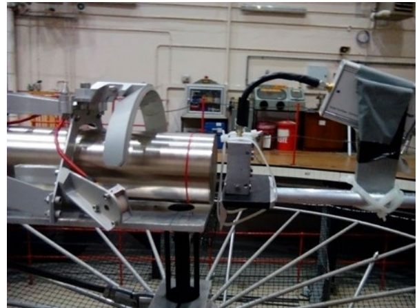
Figure 1: Experimental configuration for the determination of the neutron emission properties. NG tube is seen on the left side and the box containing the diamond detector is directly in front of it.
