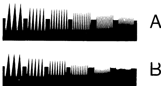
Fig. XXV-4. High-contrast renditions of the triangular-wave patterns photographed at a distance using (A) a high-quality lens, and (B) an inferior lens.
