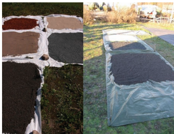
Fig. 3. Gravel setup in Nuuksio, Jul. 2007. Clockwise from top left: crushed redbrick (C Brick), sandblasting sand (Sand01), black gabbro (Gabbro), crushed LECA (LECA), and sandblasting sand (Sand05). Right: gravel samples in Espoonlahti, Dec. 2007 campaign, from top downward: Gravel, Quartz, Diabase and LECA (Kaasalainen et al. 2008b)
