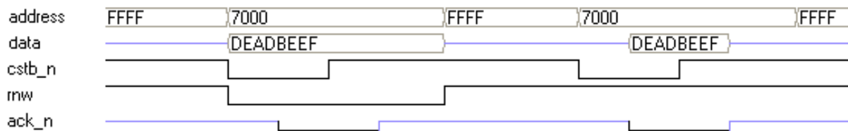
Figure 3-5: DCS bus protocol. First 0xDEADBEEF is written to register 0x7000, and then it is read back afterward (From simulation).
