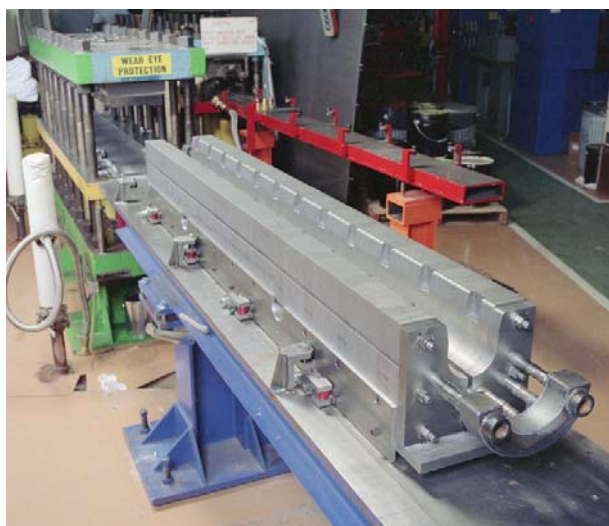
Fig. 5. A mold section made from lamination. The coil fits in the bottom and a second piece of the mold comes down from above. The pipes carry hot liquid to heat the mold and cure the epoxy.
