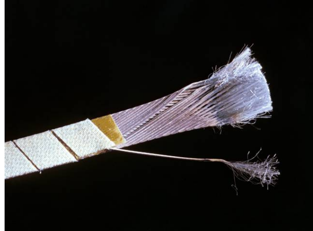
Fig. 4. The cable developed for the Superconducting Super Collider showing the epoxy impregnated glass tape, the Kapton insulation and the filaments that have been exposed by etching.
