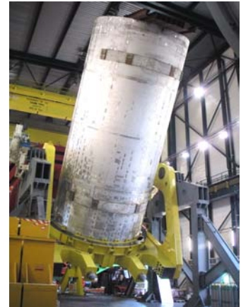
Figure 1: Swiveling of inner vacuum tank to vertical position in SX5
