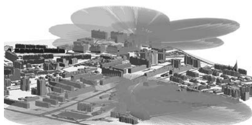
Fig. 5. Rays of radio wave propagation generated by antennas
