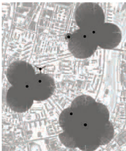
Fig. 4. Arrangement of antennas and ray propagation in experimental locality
