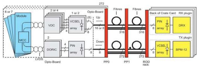
Fig. 3. Optical communication between modules and off-detector readout electronics, [2].
