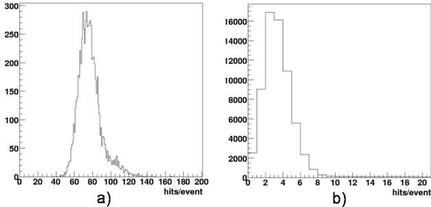
Fig. 7. Number of hits per event before a) and after b) masking of pixels with a noise occupancy above  $10^{-5}$ . The readout window is 200 ns.
