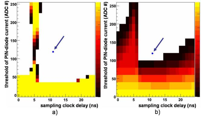
Fig. 5. Scan of the RX plug-in parameter space for the determination of an error-free region (white area) for the optical tuning. The number of bit errors is color-coded. A half-clock data pattern is used for each scan point in a) and a pseudorandom data pattern in b). The non optimal operating point chosen by the tuning algorithm is shown by the blue dot marked with the arrow.
