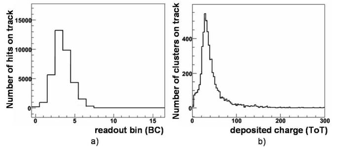
Fig. 8. Number of hits on tracks as a function of position in readout window a) and the ToT distribution of clusters on tracks b).
