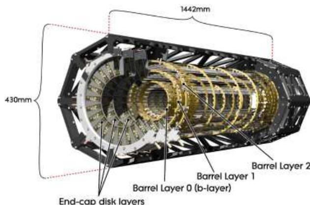
Fig. 1. View of the ATLAS pixel detector, [2].
