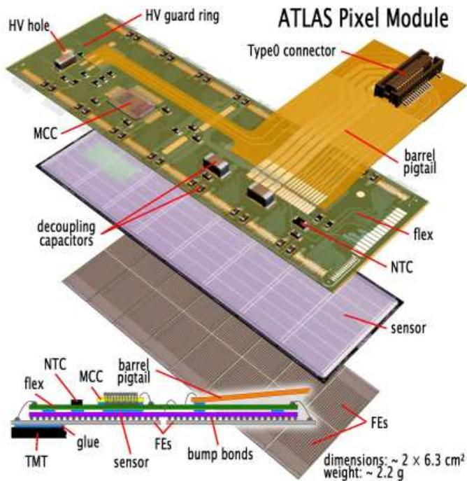
Fig. 2. Components of the pixel barrel module (disk modules have no pigtail), [2].
