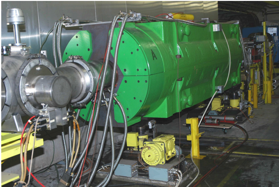
Figure 6.18: SPS high energy internal beam dump (green block) with SEM and IC on a chariot below (lower right corner). The beam impacts on the left side of the dump block.
