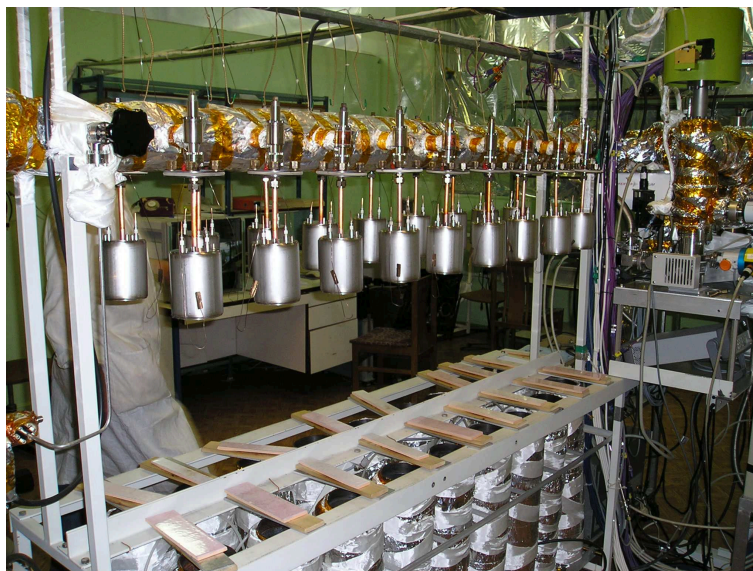
Figure 5.5: Vacuum production stand in IHEP Protvino with 18 SEMs equipped by temperature probes before pumping.
