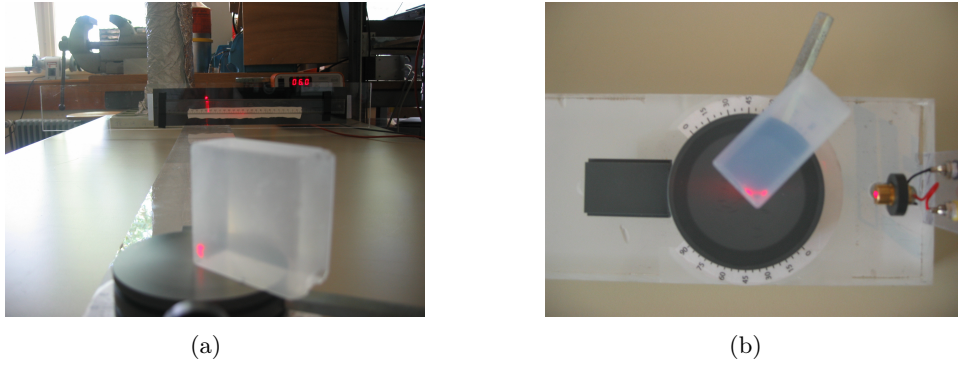
Figure 3.4: Setup for the refractive index measurement. (a): The laser crosses the aerogel and its deflection is measured. (b): Top view of the laser diode and the tile of aerogel on the rotating table.
