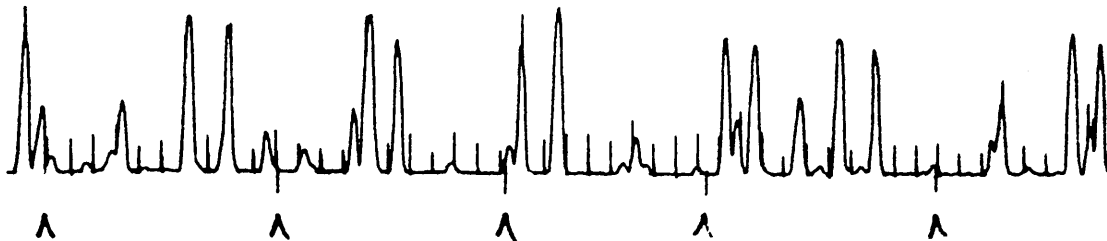
Fig. IV-3. \text{I}_2 absorption spectrum showing frequency markers.
