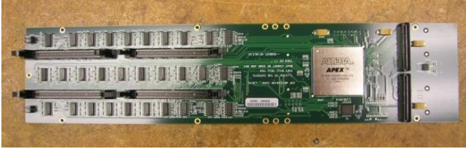
Figure 5: The actual L2CAL LVDS mezzanine card.
