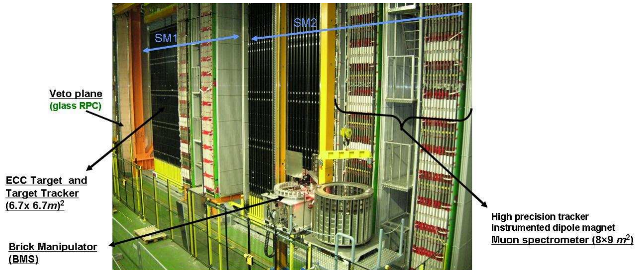
Figure 1: View of the OPERA detector in Hall C of the Gran Sasso Underground Laboratory in May 2007.
