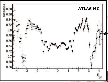
Calorimeter response  $p_T(reco)/p_T(truth)$  for jets at EM scale reveals significant variations with  $\eta_{jet}$  (cracks and dead-material regions...)
