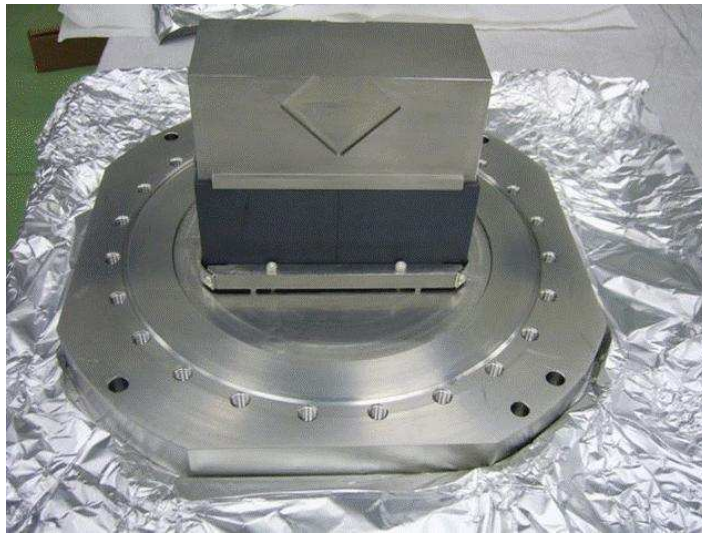
Figure 4.1: The pot with the thin window. The lateral sides of the window are 0.5 mm thick, while the bottom is 0.15 mm thick to reduce the insensitive space between the beam and the detectors inside the pot. The Ferrite collar (black in the figure) is needed to reduce the beam coupling impedance.
