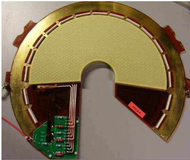
Figure 3.12: The TOTEM T2 GEM detector without front-end electronics and cooling pipes.
