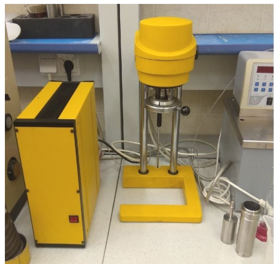
Fig.1. General view of the viscometer Rheotest RN 4.1
