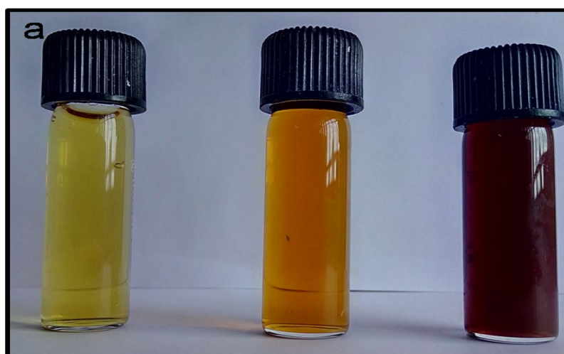
Figure S1. Green synthesized nanoparticles colour change observed from pale yellow to dark yellow then finally to red-dish brown.
