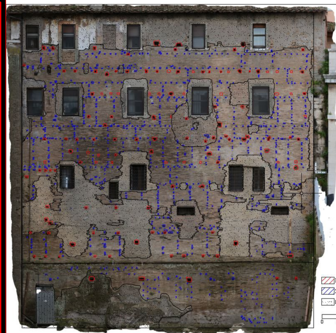
AutoCad scale line drawing of wall holes with later construction (K. Jones)
