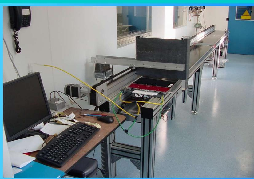
For validation of the production process, the modules produced so far are subjected to a test using a radioactive source. A Sr<sup>90</sup> source emitting electrons up to about 2.3 MeV is moved along the sense wires in 1 cm steps. For every step the wire currents are measured.
