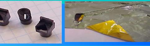
In addition wirelocators inside the straw tubes, both straw tube ends are equipped with endpieces to support and center the wire. All pieces are carefully designed not to obstruct the gas flow. The design is optimized for manufacturing in large quantities through injection moulding.
