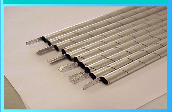
Detectors used in an LHC experiment need to be fast given that the time between consecutive bunch crossings is only 25 ns. When accepting a drift-time window of 2 or 3 bunch crossings, the speed demands can be met by using straw tubes with an inner diameter of 5 mm operated with an Ar-CO<sub>2</sub> mixture as drift gas.
