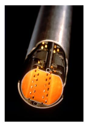
Figure 3.3.7 LHC beam pipe and beam screen with the supporting ring.
