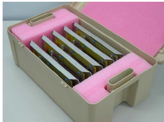
Figure 4: Transport box, fitted with only five modules. Full capacity is nine modules. The aluminum cradles of the modules snugly fit into narrow slots cut in the pink Styrofoam padding. In this picture, these slots are more clearly visible in the right-side pink foam pad.
