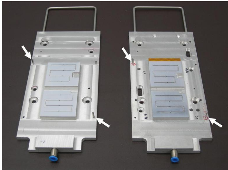
Figure 11: Bonding jigs for TIB modules with “r-phi” geometry (left: for back repair; right: for regular operation). Overall size of each jig is approximately 25 x 10 cm excluding the handle. White arrows indicate positioning pins, inserted in appropriate holes of the jig, used to lay the modules on the jig in a quick and repeatable way.
