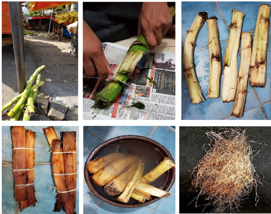
Figure 1. Banana peduncle, peduncle skin cleaning, peduncles under the retting process and extracted fibers
