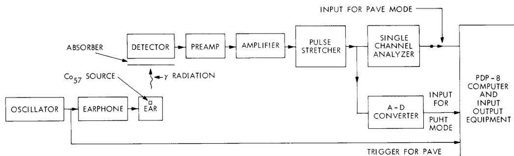
Fig. XXVII-1. Block diagram of the system.
