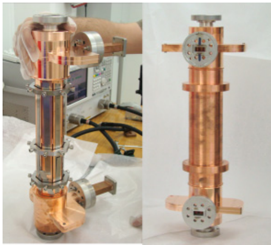
Figure 3: The 11.424 PETS during RF test (left) and before the last EB welding (right).
