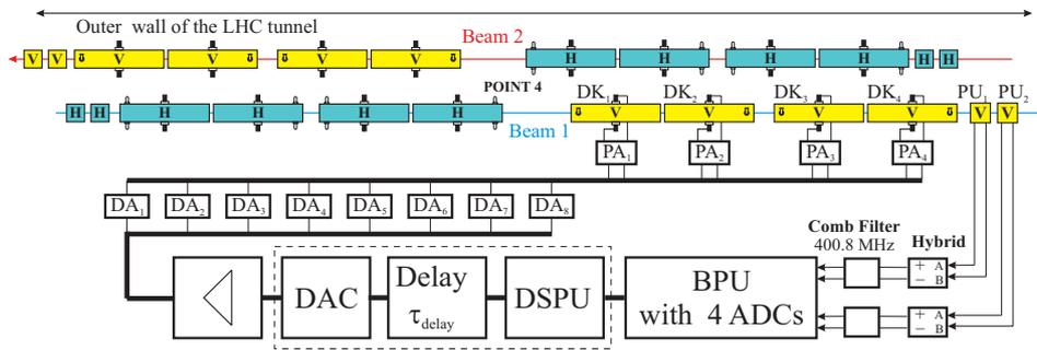
Figure 1: Layout of the LHC Damper and block diagram of the transverse feedback system for vertical oscillations.
