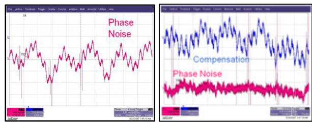
Figure 8: Klystron Phase Ripple (10mV/deg): Left Polar loop off, scale 10mV/div. Right : Loop on, scale 2mV/div.
