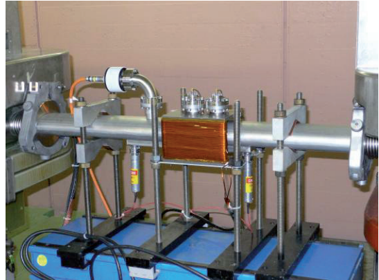
Figure 1: Picture of the PS electron cloud experiment comprising a fast vacuum diagnostic, shielded button pickups, a dipole magnet, and a clearing electrode.
