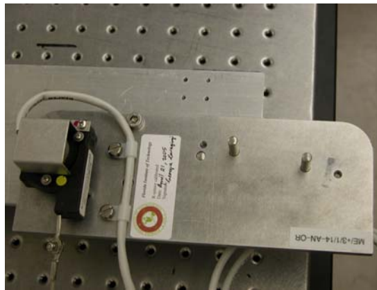
Figure 2.26 The main sensor mount with one R1 sensor on plate ME+3/1/14-AN-OR is positioned by means of two dowel pins and a spacer on a stand.
