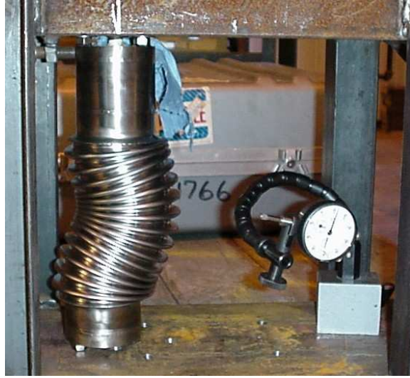
Figure 4.4: “Squirm” test of a bellows unit. Squirm occurred at 190 psi (13 atm).
