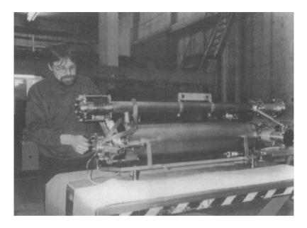
FIGURE 7 A nine-cell cavity is welded into the LHe tank (lower cylinder). The cold end of the input coupler is visible at the right end, the tuner is assembled at the left end, the LHe line is shown on top of the structure.
