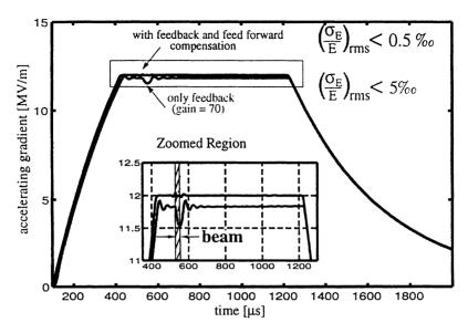
FIGURE 12 Cavity voltage during pulsed operation with beam. The fluctuation of the cavity voltage is smaller 5% with feed back and reduced to smaller 0.5% with additional feed forward compensation.
