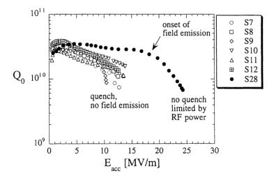
FIGURE 4 Performance of 6 cavities from one vendor: decrease of the Q value at low gradients (but no field emission) and early thermal breakdown between  $E_{\rm acc}$  10 and 14 MV/m. The defects were localised at the equatorial welding and could be traced back to improper cleaning and not optimised welding parameters. One more cavity was fabricated with improved fabrication conditions and showed excellent performance (S28).
