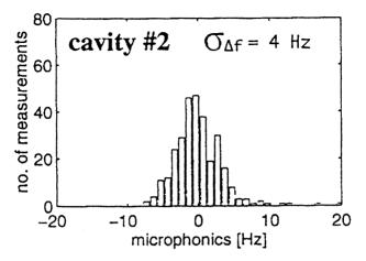
FIGURE 13 Result of the search for microphonics: the resonance frequency of a cavity in the module is measured and statistically evaluated. No microphonics is present because the frequencies are centred around the nominal value.
