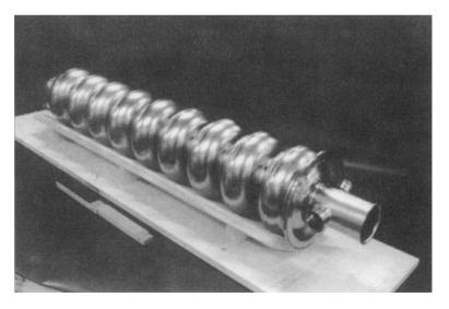
FIGURE 2 Nine-cell TTF cavity. On the right beam pipe the port for the input coupler (front side) and the HOM coupler (back side) can be seen.
