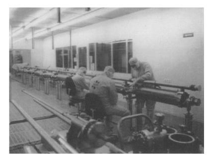
FIGURE 8 Assembly of a string of 8 nine-cell cavities and one quadrupole during handling in the clean room.
