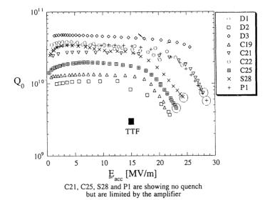
FIGURE 3 Performance of "good" cavities in the vertical measurement. Four cavities (C21, C25, S28, P1) were limited by available RF power. The typical decrease of the Q value at high gradients is due to field emission.
