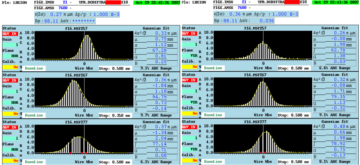
Figure 4.8: Horizontal (left profiles) and vertical (right profiles) SEM-wire measurements in TT2 at 5.88 GeV/u. Normalized r.m.s. emittances: \epsilon_H^* = 0.49 \mu\text{m} , \epsilon_V^* = 0.65 \mu\text{m} ( \beta\gamma = 7.246 ).
