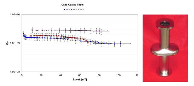
Figure 4: 2.8 GHz prototype crab cavity for the APS and its Q vs. peak magnetic field plot from JLab tests.
