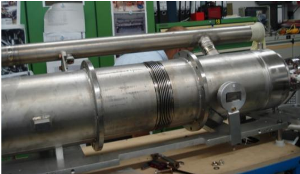
Fig. 36 – Z86 and modified He tank with support disks and bellow, ready for Blade tuner installation
