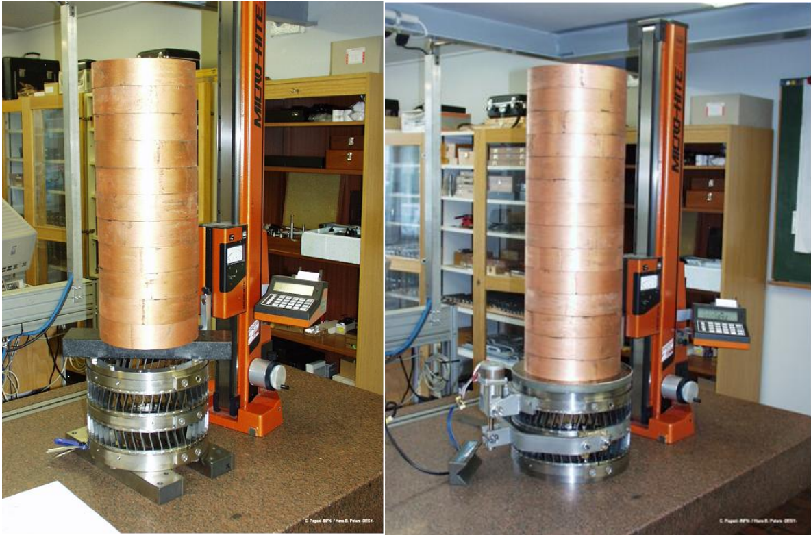
Fig. 4: Pictures of experimental compression tests on blade tuner, showing both the experimental configurations.
