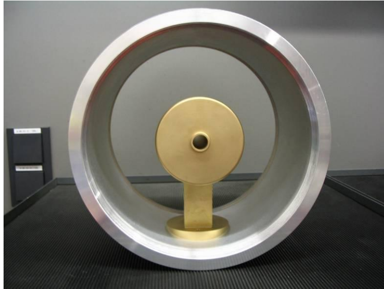
Fig.18: A detail of the incoupling cell including the dummy triplet
