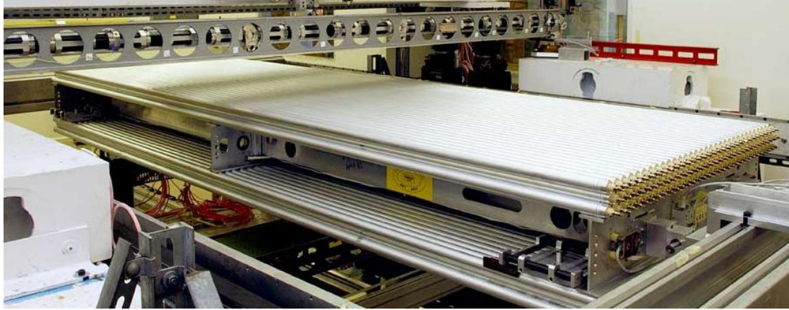
Figure 14: A view of a MDT chamber. Two groups of 3 monolayers form a multilayer.
