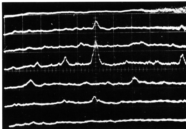
Fig. XXX-14. Response of system to noise-free input; 5 bits/cm horizontal, arbitrary intensity (each trace) vertical; the traces correspond to equidistant channels in the output plane.
