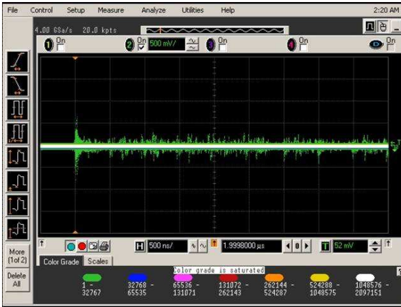
Figure 3 Oscilloscope trace showing a test for voltage spikes. The trace was taken in persistency mode for 12 hours with -140V applied. The voltage scale is 500mV/div. The time scale is 500ns/div.
