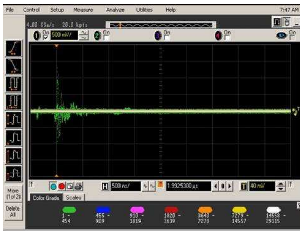
Figure 12 Oscilloscope trace of the output voltage during a brown-out when it is in persistency mode. The voltage scale is 500mV/division. The time scale is 500ns/division.
