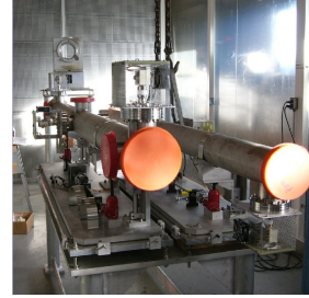
Figure 5.2: The two RHIC BBLRs before installation
