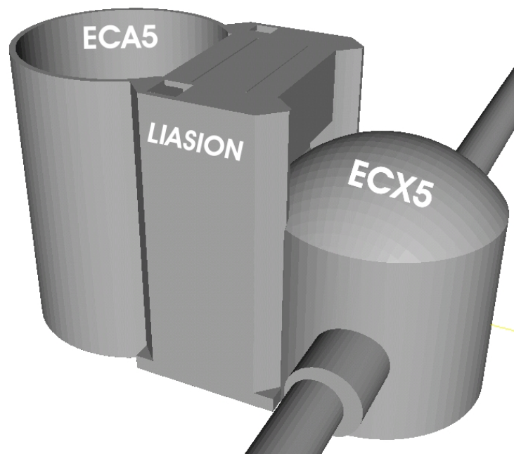
Figure 6.1 The SPS5 underground constructions consist of the assembly area ECA5, the experimental area ECX5 and the liaison area including 20 crossing zones.
