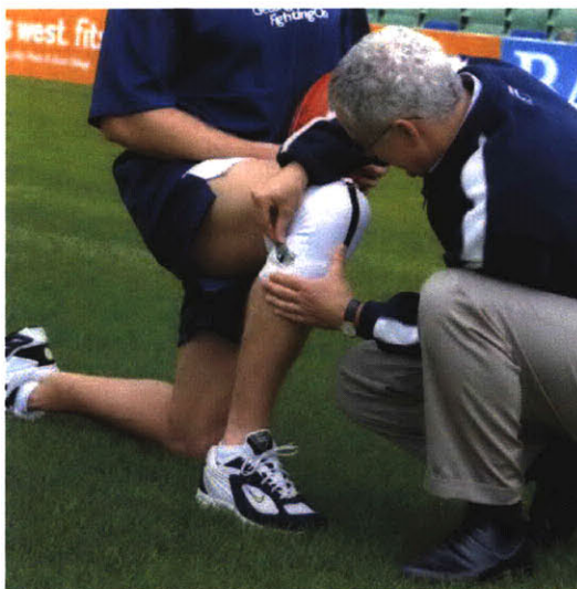
Figure 3-1: The Intelligent Knee Sleeve uses PPy-coated fabric as a strain gauge to monitor the wearer’s knee joint motion. Image by CSIRO Textile and Fiber Technology (Taken from [13])
