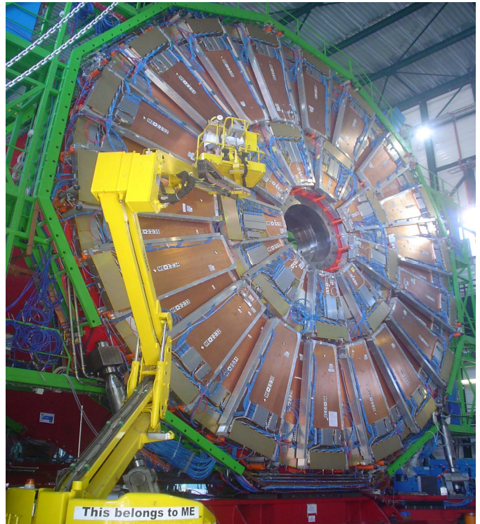
Fig. 2. Fully instrumented CMS Muon Endcap station ME+2. Note the inner and outer rings of cathode strip chambers with overlaps between chambers in \phi .
