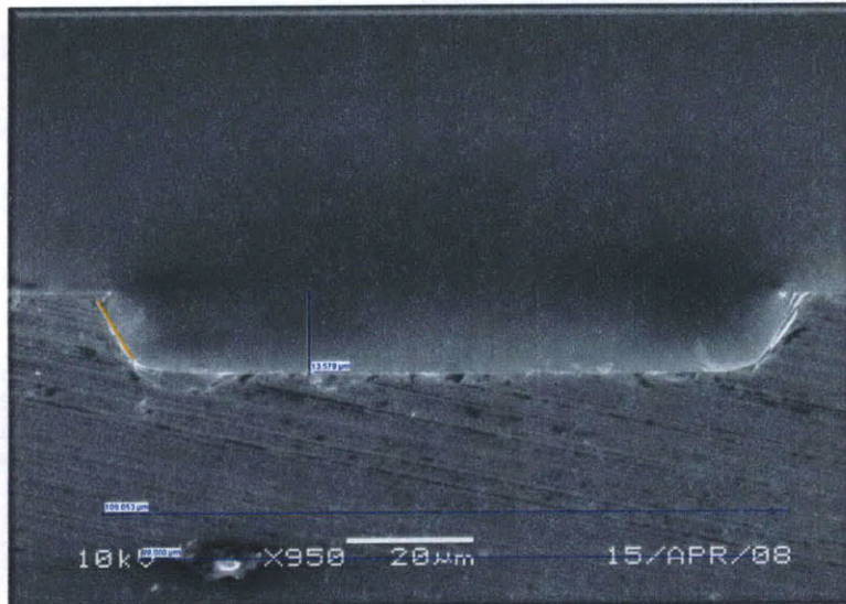
Figure 6.6 – The sidewall profile for a feature with very small aspect ratio; the sidewall is straight.
