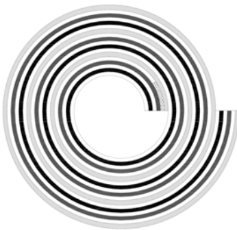
Figure 6: Schematic of a switch (not to scale) showing the non-inductive bifilar HTS winding co-wound with a resistive heater and insulation. The current and voltage terminals, support, and outer insulation/heater section have been omitted for clarity. White regions represent insulation, black the heater, and light and dark grey the HTS which were soldered together over the crossed region.
