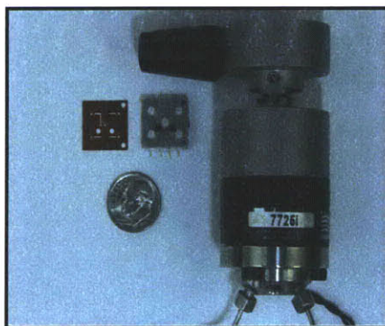
Figure 5.12: 5-valve manifold shown in size comparison to the HPLC valve it replaced.
