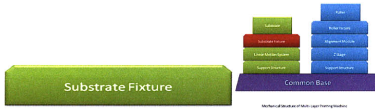
Figure 4.29 Substrate fixture will define substrate's position.
