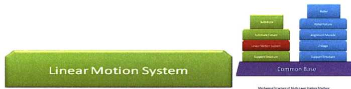
Figure 4.28 Linear motion system conveys the substrate and its fixture.
