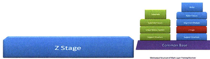
Figure 4.30 Z stage is used to move its upper component vertically.
