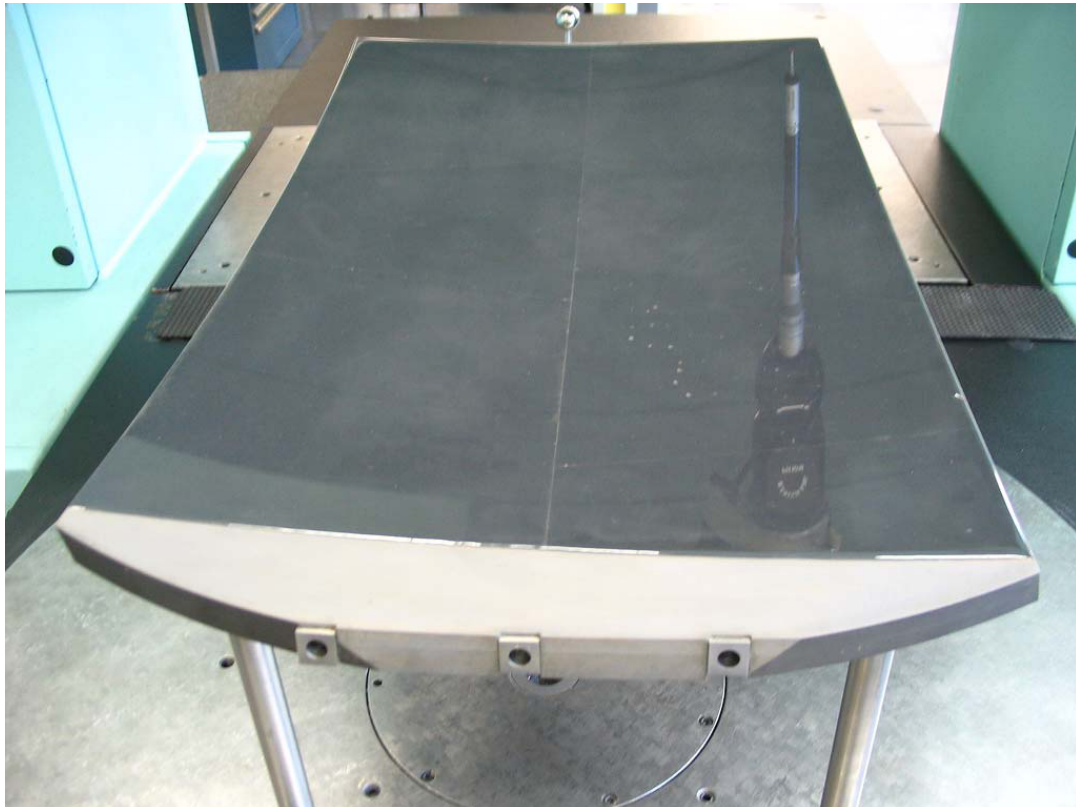
Figure 5.5: A view of the mirror showing the three titanium inserts and the glass coating.
