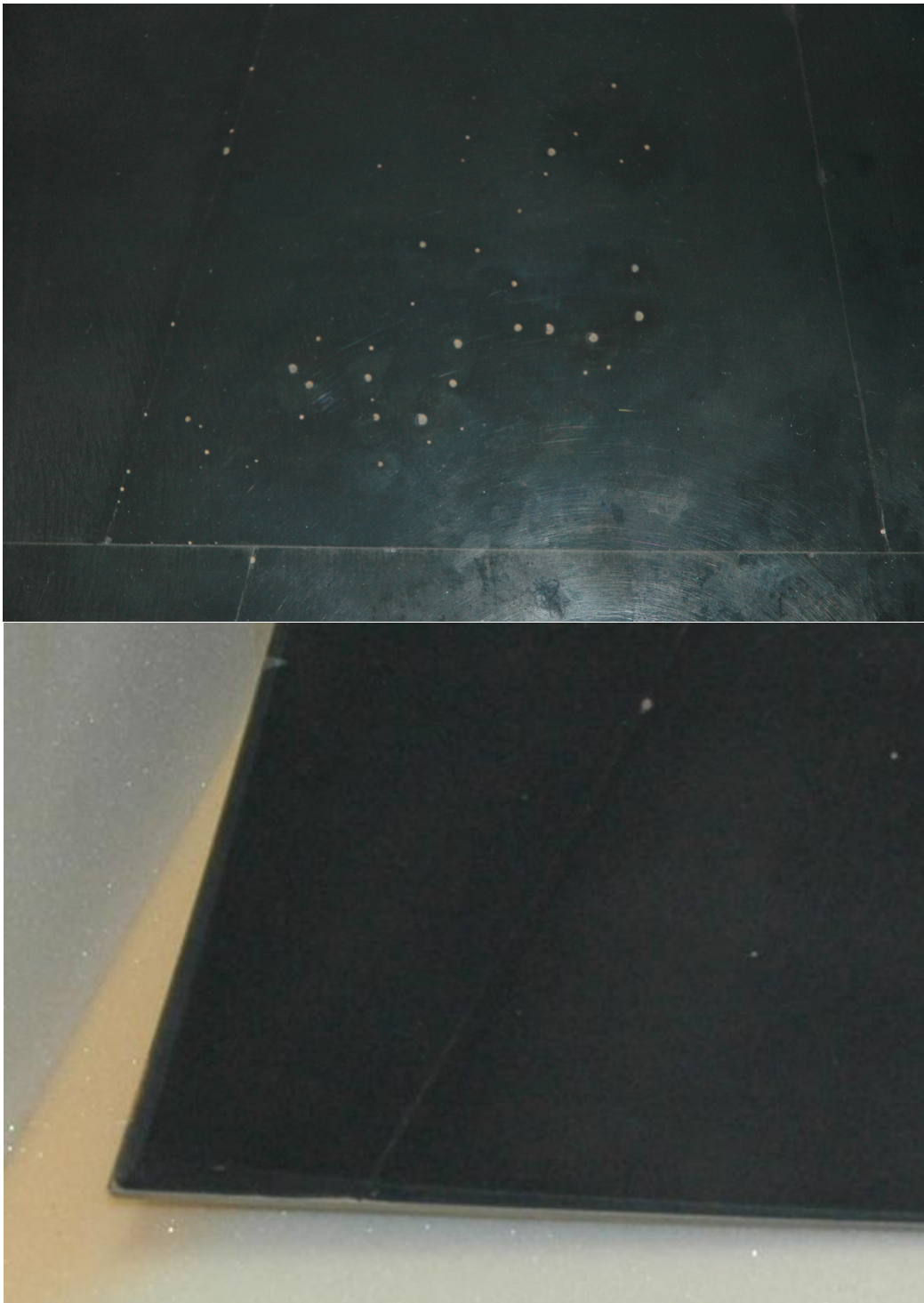
Figure 5.6: The optical surface of the glass-coated beryllium mirror showing the two causes of optically-dead areas: pits in the glass layer (upper image) and the large chamfer due to the correction of the substrate's radius of curvature (lower image). The pits are confined to the boundaries between the glass segments and the centre of one particular segment. The large chamfer is only present at the edges of the mirror farthest from the mount point.
