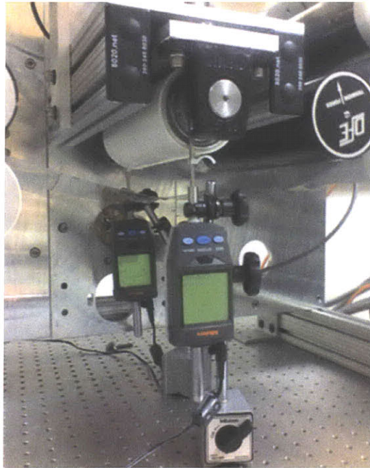
Figure 55: Setup for The Repeatability of the Parallelism Test
